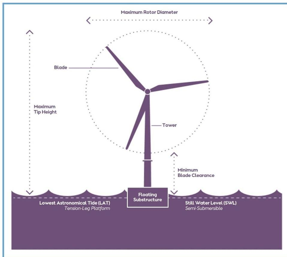
Figure 4-4 Indicative Floating Wind Turbine Generator.
