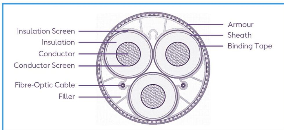
Figure 4-12 Indicative Cross-Section through an Offshore Cable
