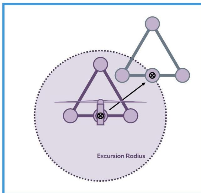
**Figure 4-9 Floating Substructure Excursion**
