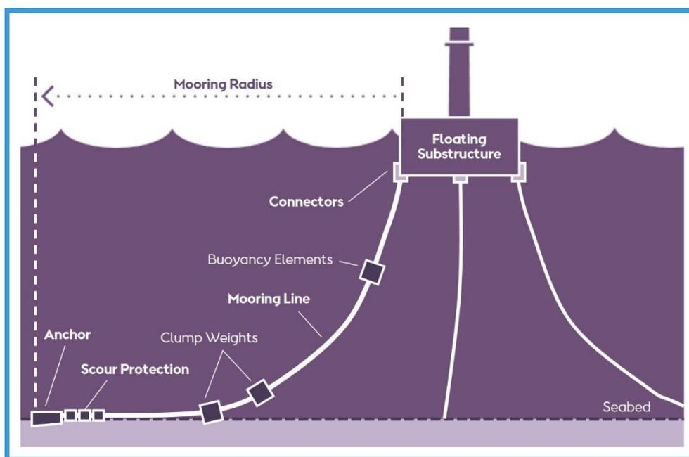
**Figure 4-8 Components of the Mooring System**
