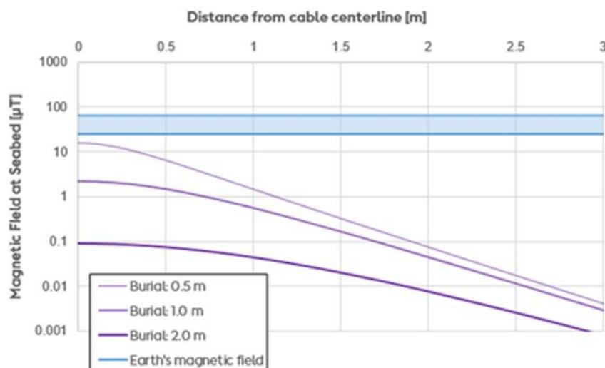
Figure 4-24 Magnetic Field at the Seabed for Buried 66 kV Cables
