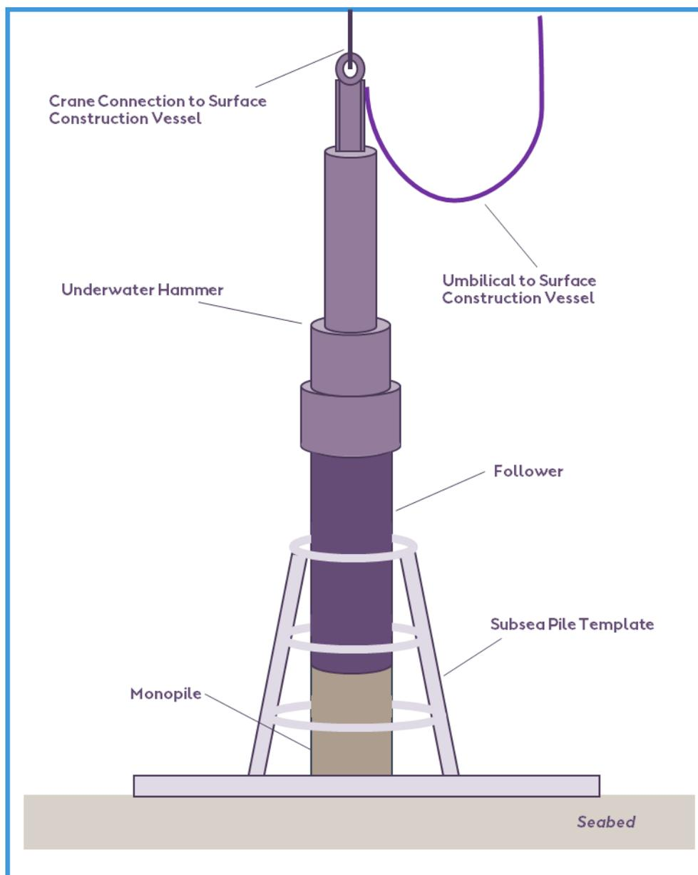
Figure 4-11 Example set-up of equipment used to drive sub-sea piles for mooring anchors
