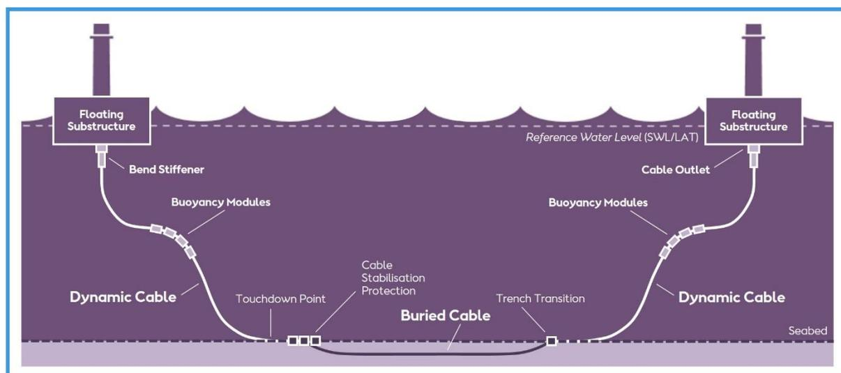
Figure 4-13 Components of the Offshore Cable System
