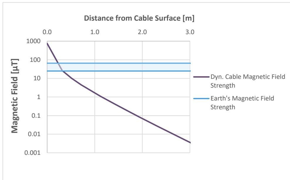
**Figure 4-23 Magnetic Field for 66 kV Cables in the Water Column**
