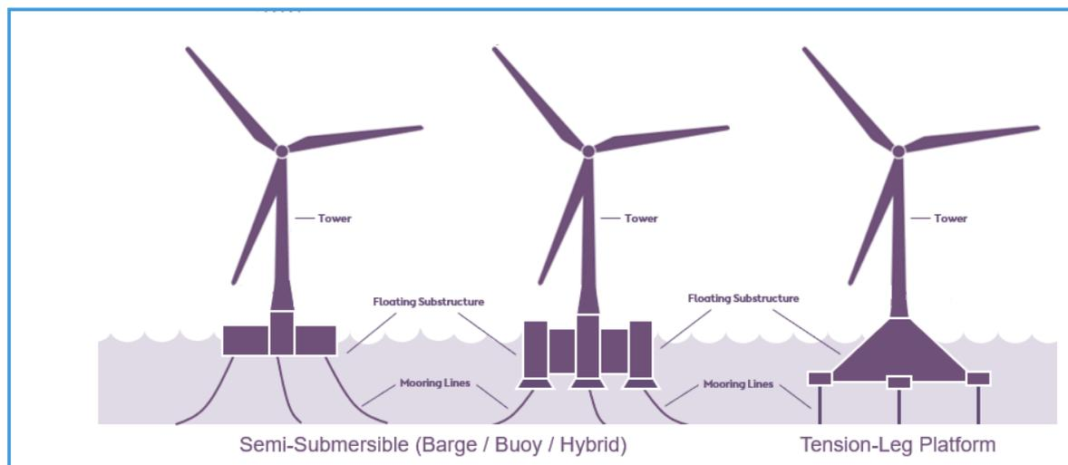
Figure 4-5 Indicative Floating Substructure Configurations
