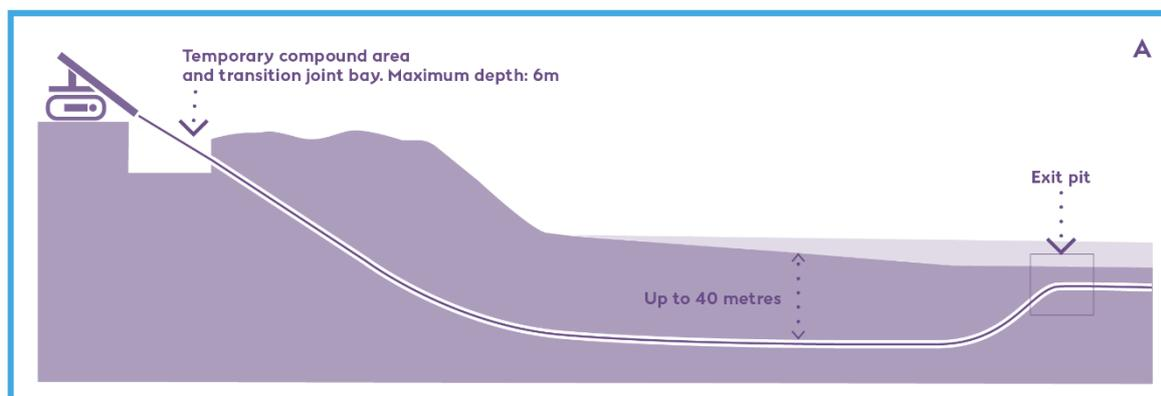
Figure 4-21 Indicative Trenchless Installation Arrangement
