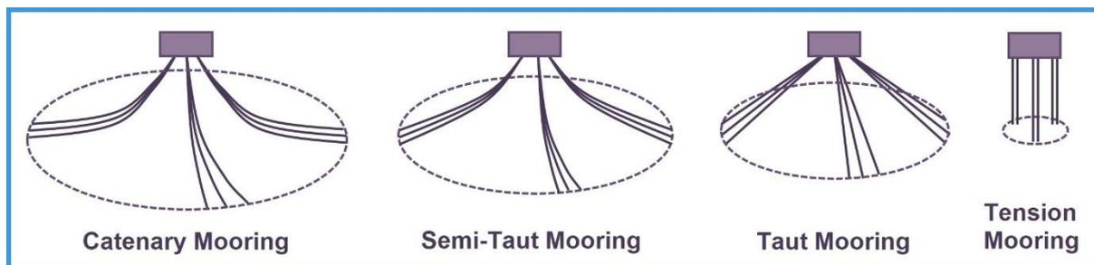
Figure 4-7 Indicative Mooring System Configurations
