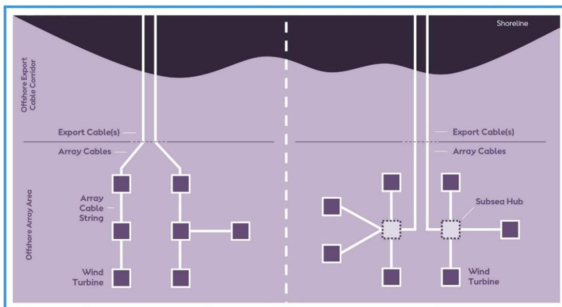
Figure 4-15 Indicative Offshore Cable Layout Configurations
