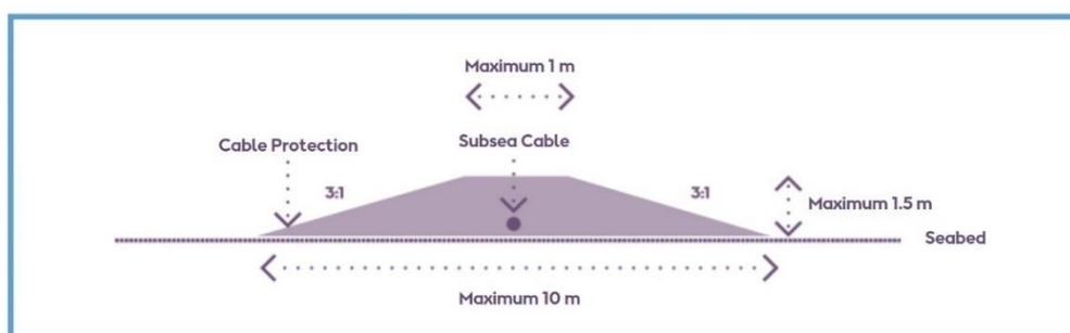
**Figure 4-16 Indicative Cable Protection Berm**
