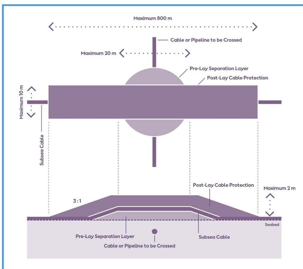
Figure 4-17 Indicative Cable Crossing Cable Protection Arrangement
