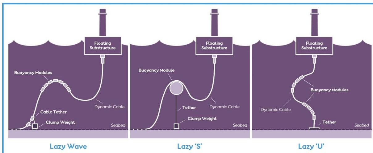
Figure 4-14 Indicative Dynamic Cable Configurations
