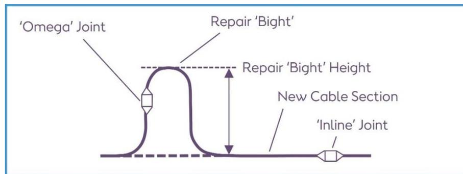
Figure 4-22 Indicative Top-Down View of a Typical Cable Repair
