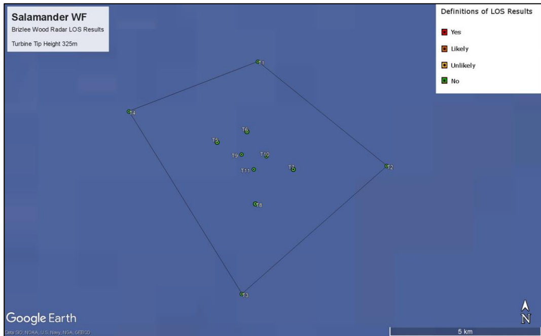
Figure 9 - Salamander Project Offshore Array Area (representative WTGs) – Brizlee Wood Radar LoS results (tip height 325m)
