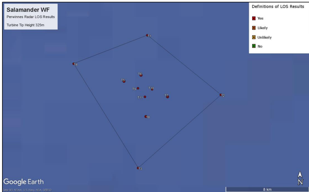
Figure 5 - Salamander Project Offshore Array Area (representative WTGs) – Perwinnes Radar LoS results (tip height 325m)
